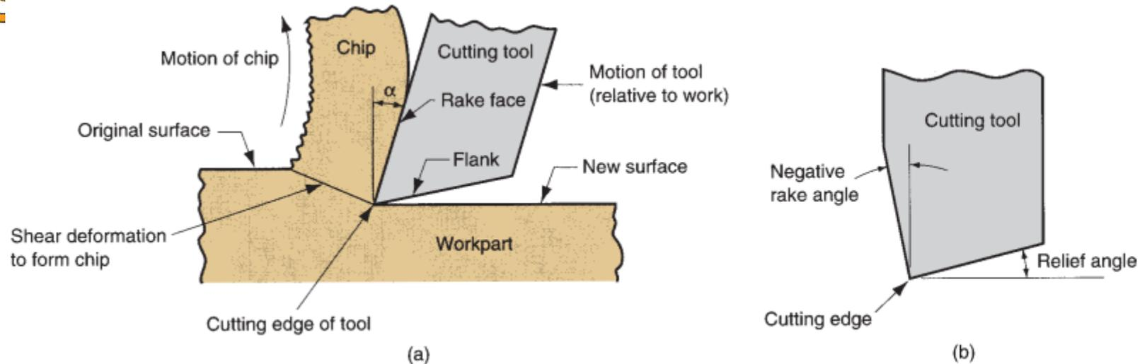
**Figure 20.2** (a) A cross-sectional view of the machining process. (b) Tool with negative rake angle; compare with positive rake angle in (a).
