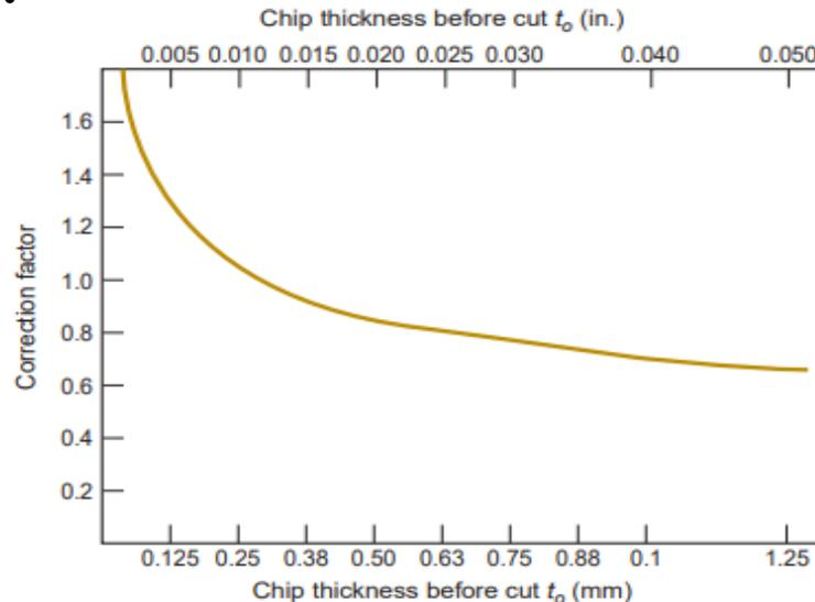
**FIGURE 20.14** Correction factor for unit horsepower and specific energy when values of chip thickness before the cut to are different from 0.25 mm (0.010 in).
