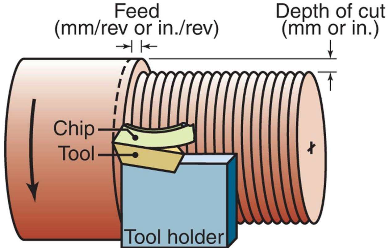
**Schematic illustration of the turning operation, showing various features.**
