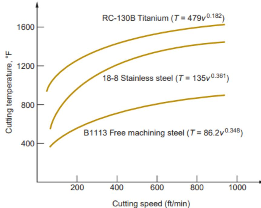
**FIGURE 20.15** Experimentally measured cutting temperatures plotted against speed for three work materials, indicating general agreement with Equation (20.23). Based on data [1].
