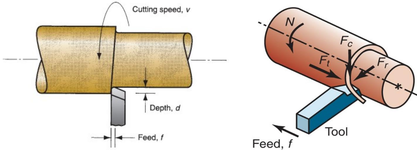
**Figure 20.5: *Cutting speed, feed, and depth of cut* for a turning operation.**
