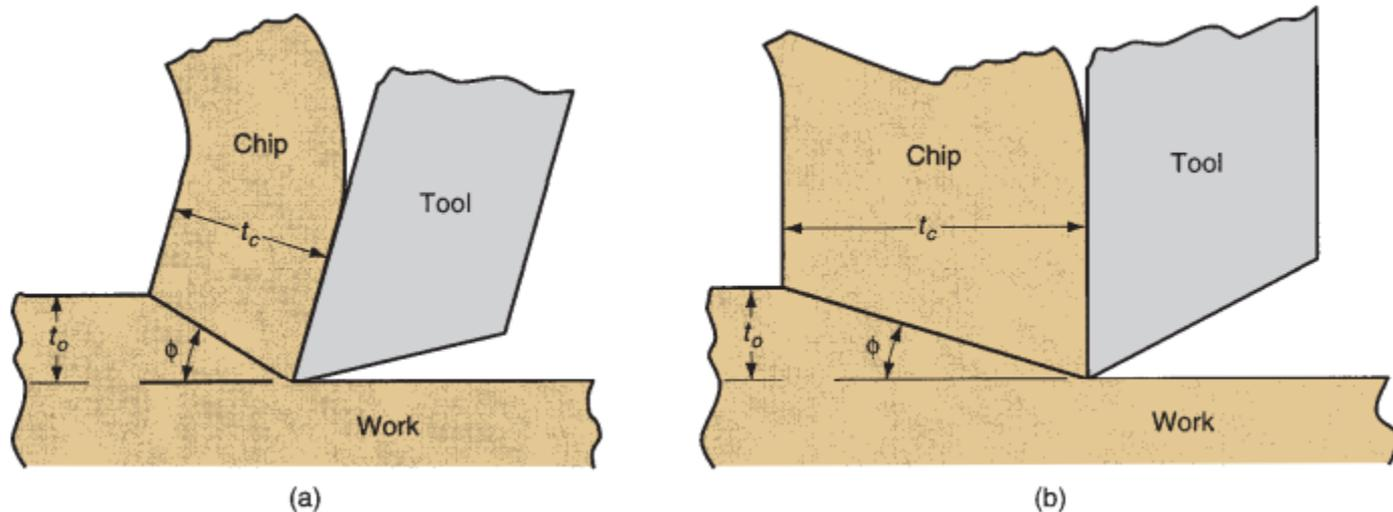
**FIGURE 20.12** Effect of shear plane angle  $\phi$ : (a) higher  $\phi$  with a resulting lower shear plane area; (b) smaller  $\phi$  with a corresponding larger shear plane area. Note that the rake angle is larger in (a), which tends to increase shear angle according to the Merchant equation.
