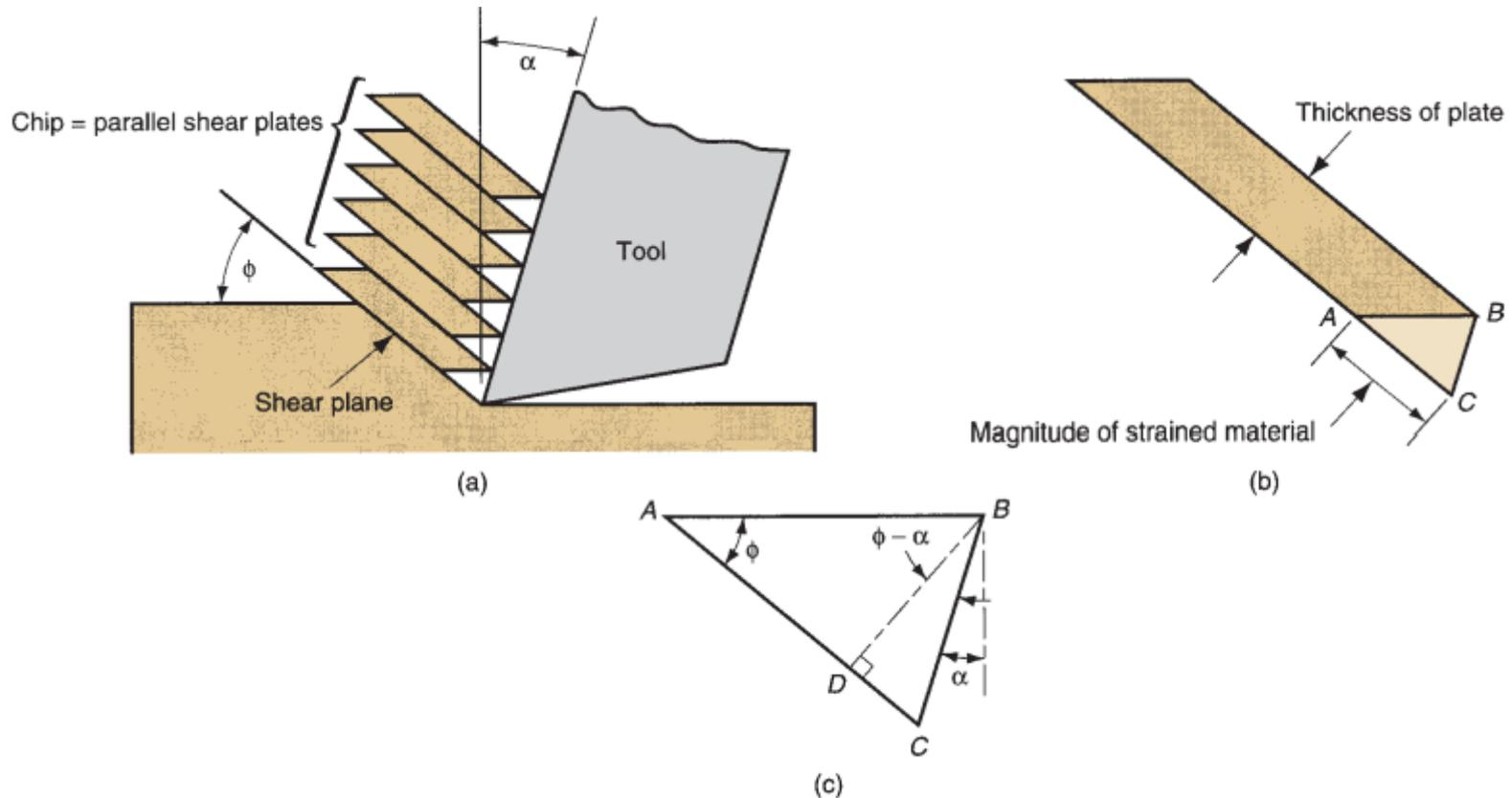
**Figure 20.7 Shear strain during chip formation:**
