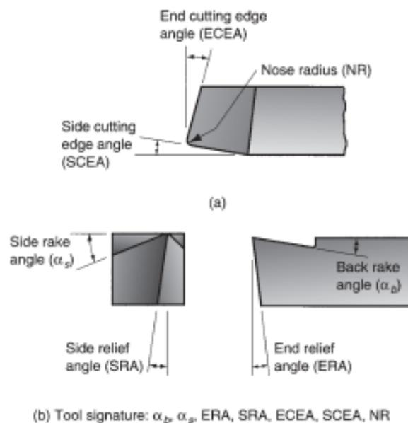
FIGURE 22.7 (a) Seven elements of single-point tool geometry, and (b) the tool signature convention that defines the seven elements.
