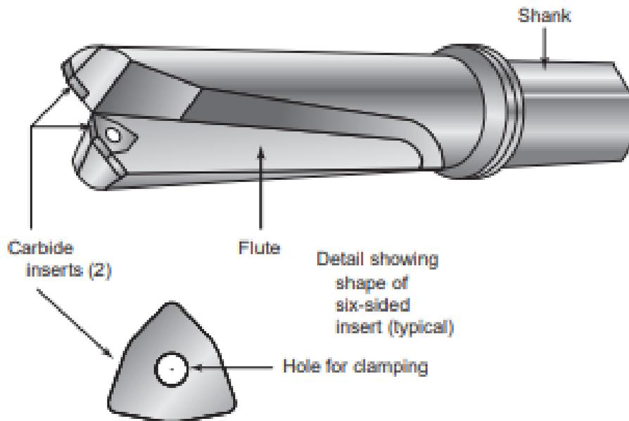
FIGURE 22.13 Straight-flute drill that uses indexable inserts.
