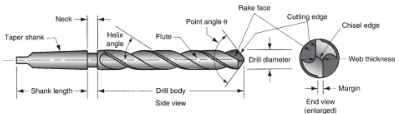
FIGURE 22.12 Standard geometry of a twist drill.
