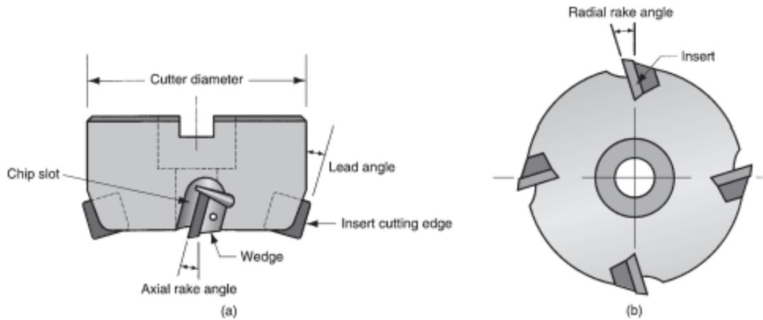
FIGURE 22.17 Tool geometry elements of a four-tooth face-milling cutter: (a) side view and (b) bottom view.
