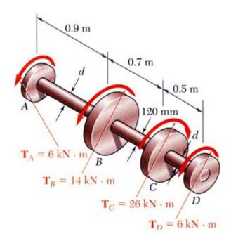
Shaft BC is hollow with inner and outer diameters of 90 mm and 120 mm, respectively. Shafts AB and CD are solid of diameter d. For the loading shown, determine (a) the minimum and maximum shearing stress in shaft BC, (b) the required diameter d of shafts AB and CD if the allowable shearing stress in these shafts is 65 MPa.
