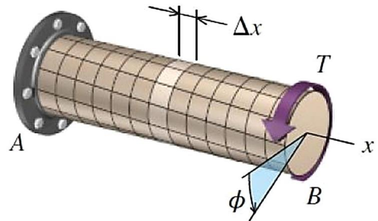
(b) Deformed shaft in response to torque  $T$
