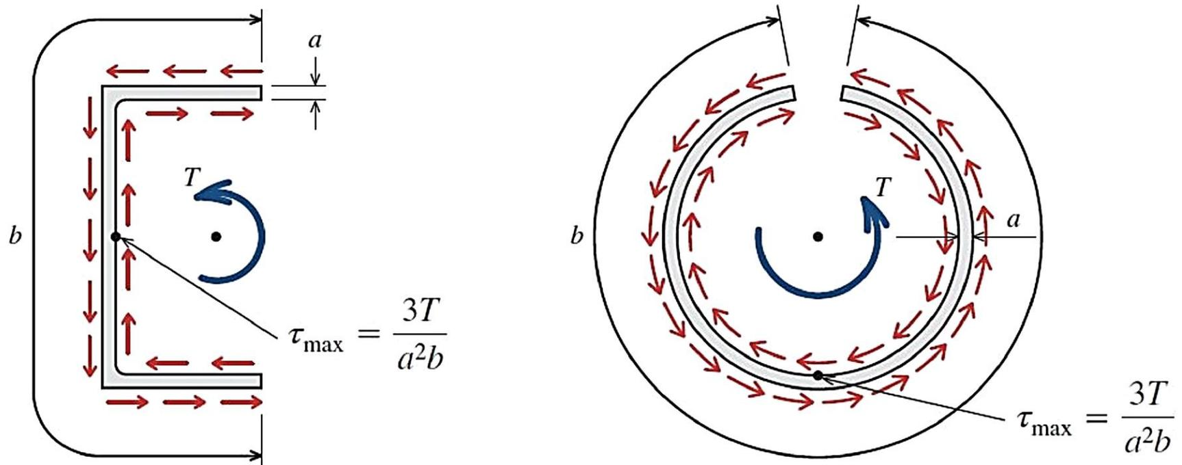
Fig 7.5: Equivalent narrow rectangular sections with shear stress distribution.
