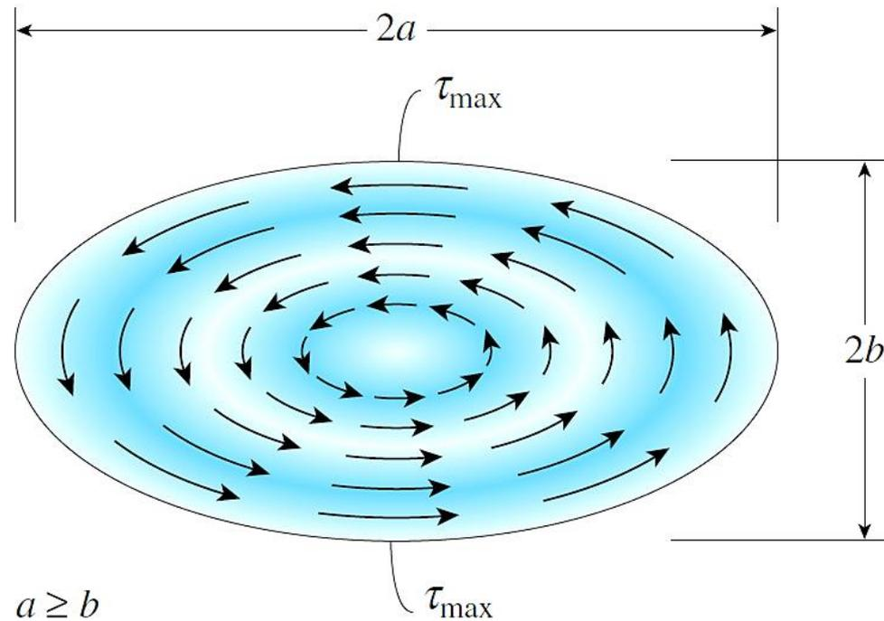
Figure 7.3.4: Shear Stress distribution in an elliptical bar
