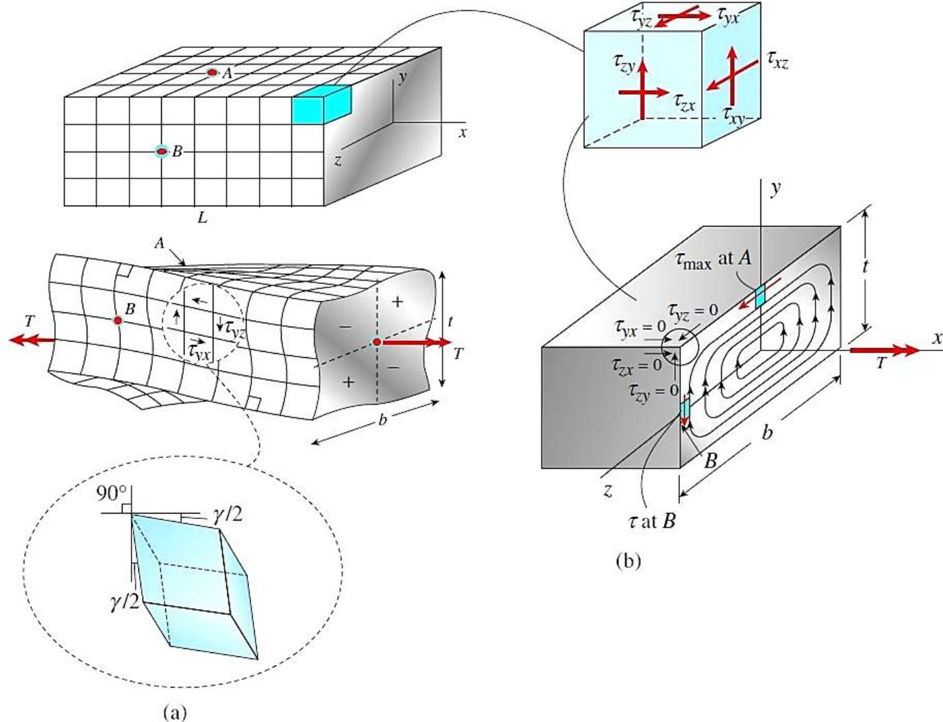
Figure 7.3.2 (a) Torsion of a bar of rectangular cross section and (b) shear stress distribution for a bar of rectangular cross section acted upon by torsional moment  $T$
