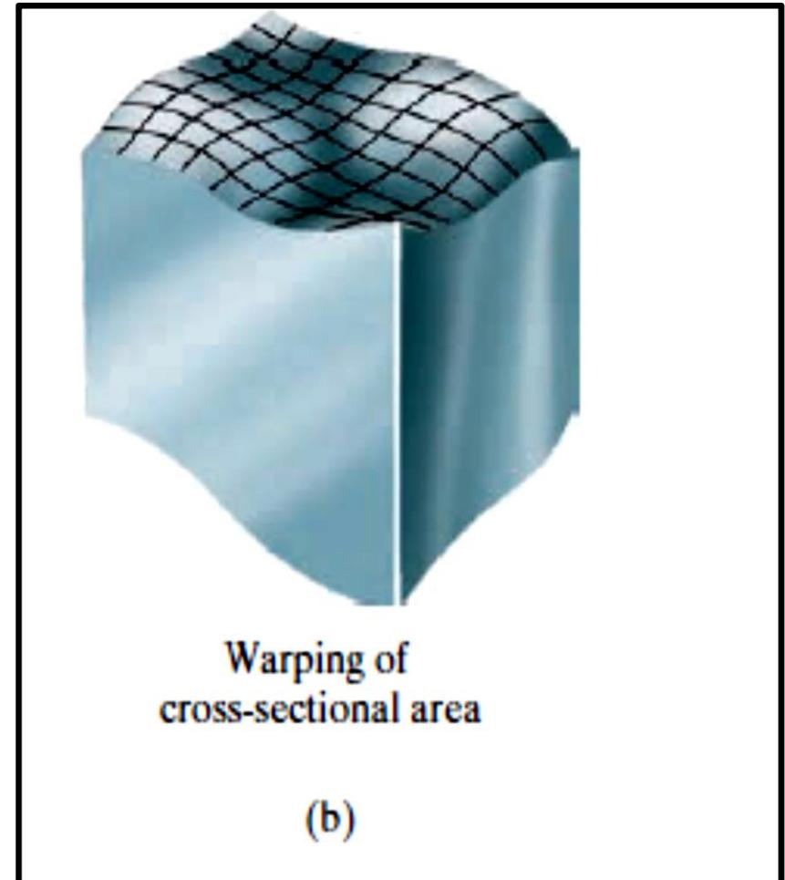
Fig. 7.3.1: Stress distribution in a square shaft
