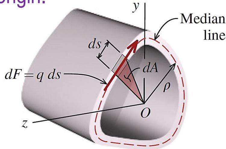
Fig. 7.8 : Relationship between internal torque and shear stress in a thin-walled section.
