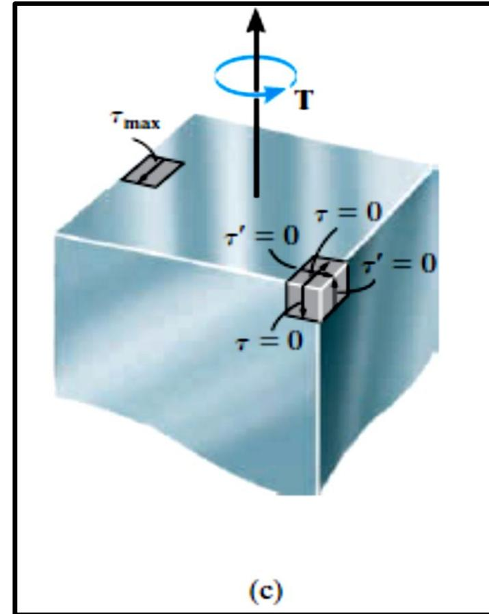
Fig. 7.3.1 (c): Stress distribution in a square shaft
