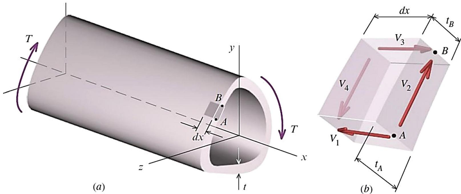
Fig. 7.6: Shear flow in thin-walled tubes.
