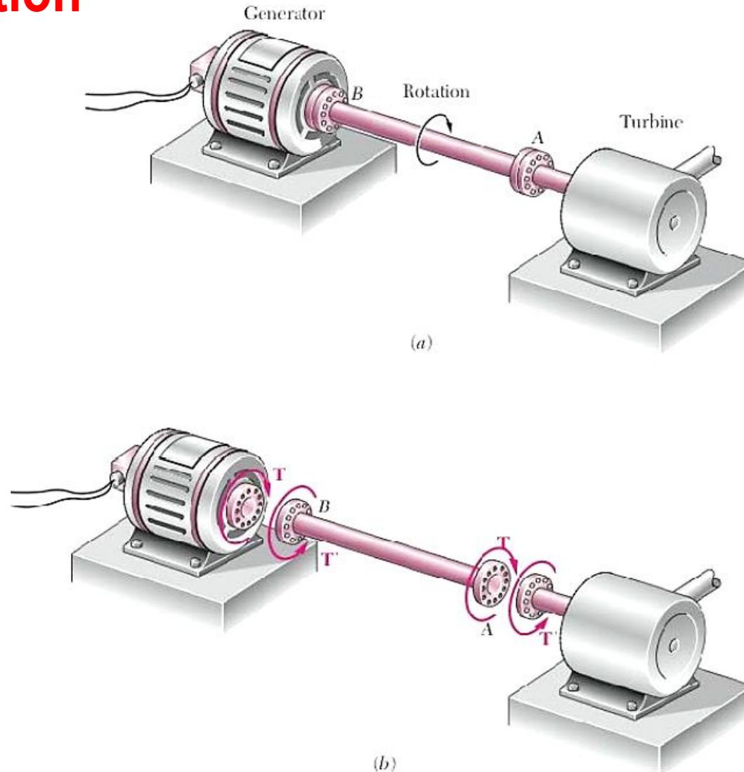
Fig.7.1 (c): Circular shaft subjected to pure torsion
