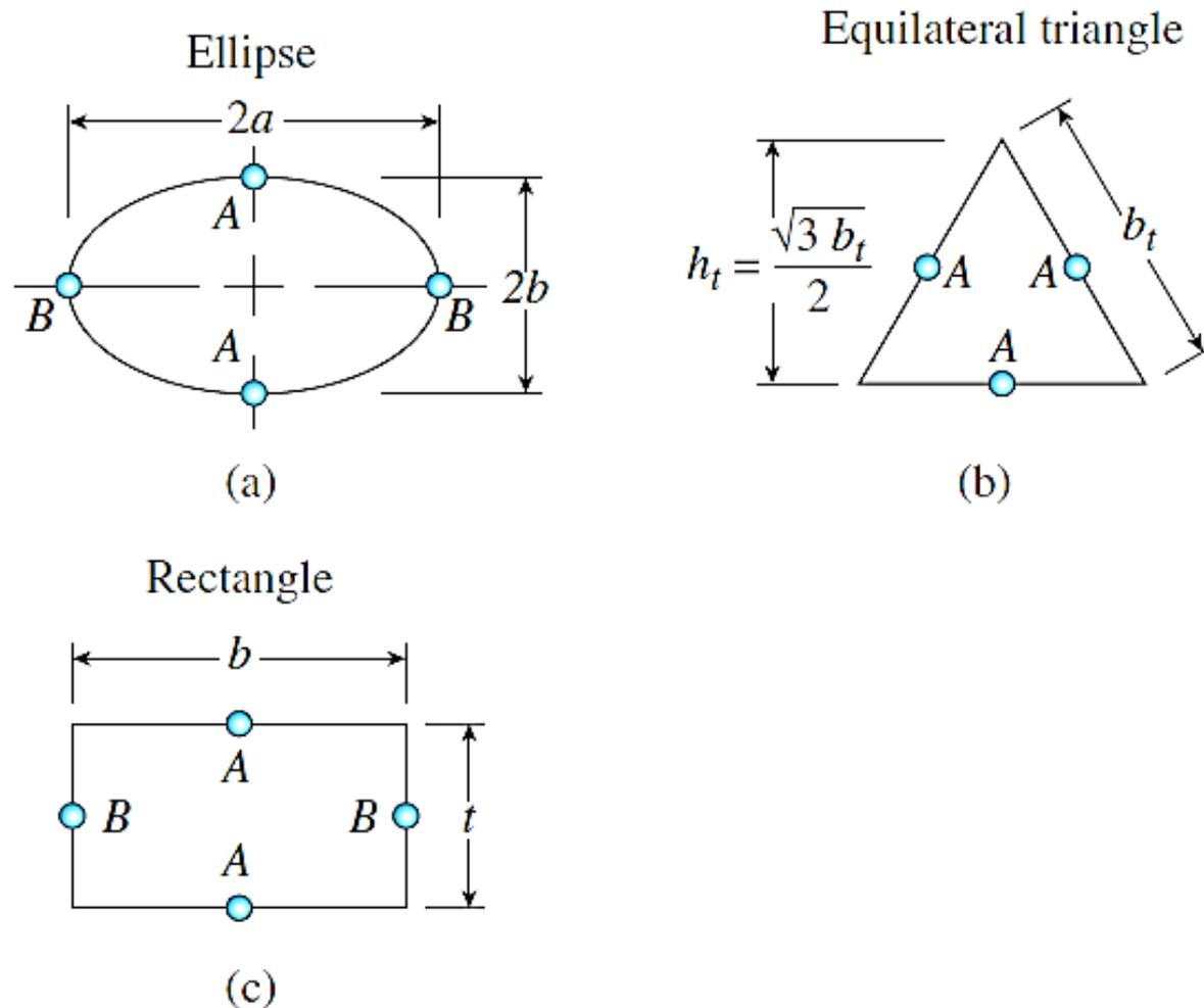
Figure 7.3.3 : Solid elliptical, triangular, and rectangular cross-sectional shapes
