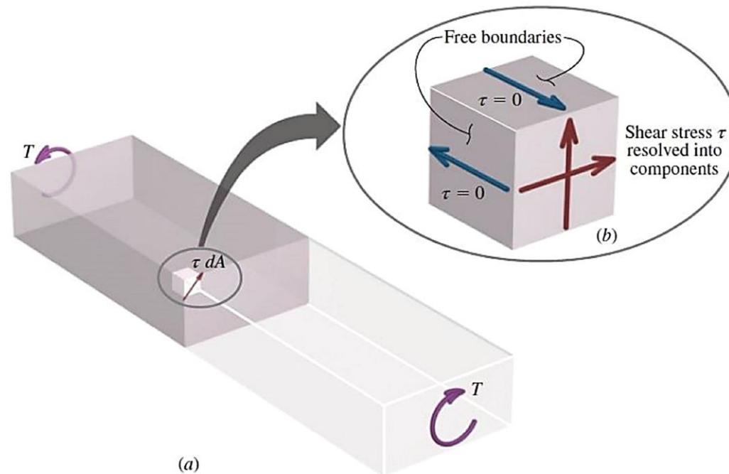
Fig. 7.4: Torsional shear stresses in a rectangular bar.
