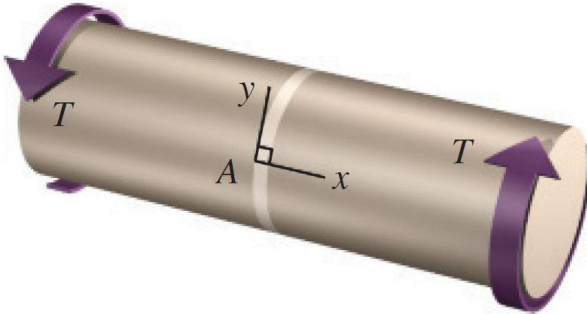
Fig.7.1 (d): Circular shaft subjected to pure torsion
