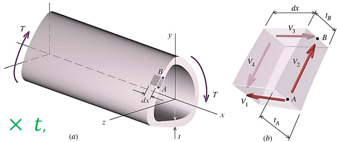
Fig. 7.6: Shear flow in thin-walled tubes.
