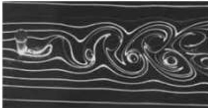
Figure 3.2 Streaklines in the unsteady flow around a cylinder. (Photograph by Sadatashi Taneda.)
