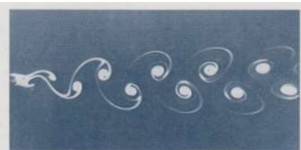
Figure 3.2 Streaklines in the unsteady flow around a cylinder. (Photograph by Sadatashi Taneda.)
