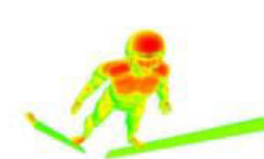
Fig. 2a. Distribution of aerodynamic drag coefficient (FLA of 20°)
