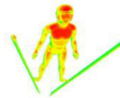
Fig. 2c. Distribution of aerodynamic drag coefficient (FLA of 40°)
