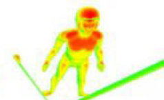
Fig. 2b. Distribution of aerodynamic drag coefficient (FLA of 30°)
