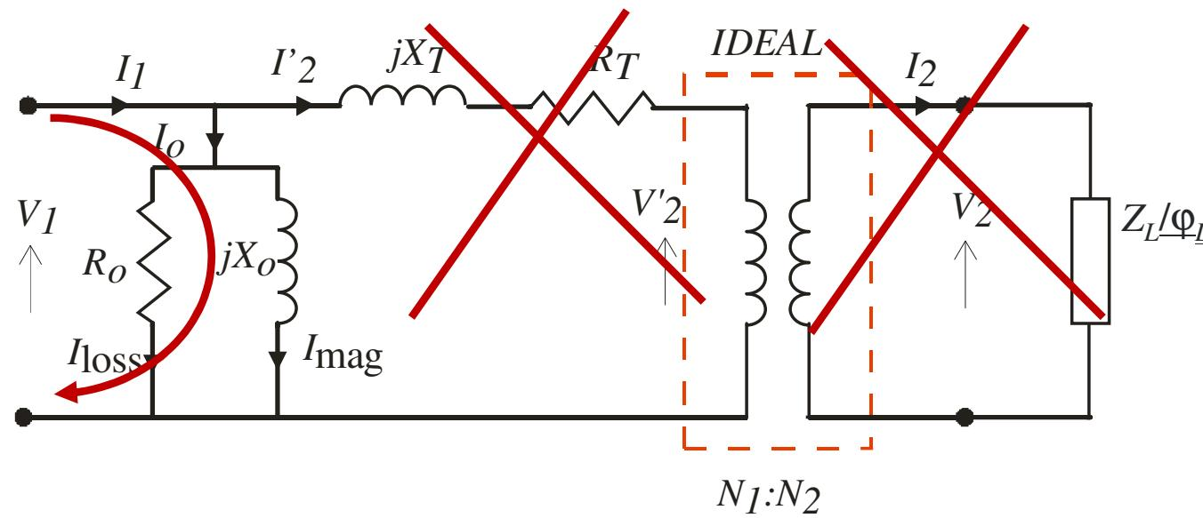
$$R_o = \frac{V_1}{I_{Loss}} = \frac{240}{0.78} = 308 \Omega$$
