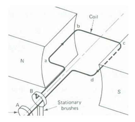
$$V_{in} = "Blu" = B(2l)u = 0.5 \times (2 \times 0.2) \times 12 = \underline{2.4 \text{ V}}$$
