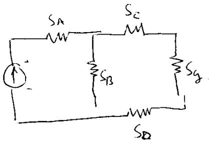
$$(a) \quad S_g = \frac{l}{\mu A} = \frac{10^{-3}}{4\pi \cdot 10^{-7} \cdot 159 \cdot 10^{-6}} = \underline{\underline{5 \times 10^6 \text{ A/Wb}}} \quad 5$$
