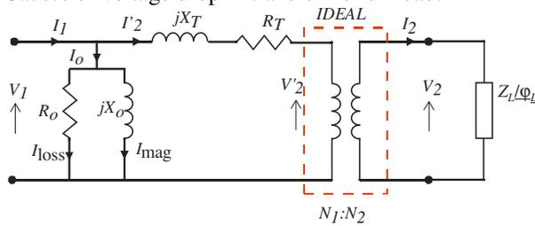
As in the equivalent circuit, the series elements  $R_T$  and  $X_T$  cause voltage drop when load current  $I_2$  flows.
