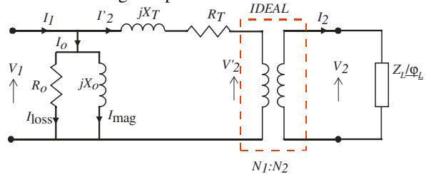
As in the equivalent circuit, the series elements  $R_T$  and  $X_T$  cause voltage drop when load current  $I_2$  flows.
