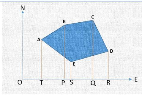
Expanding the expression leads to: **Area** =  $\frac{1}{2} \left[ \sum_{i=1}^{n} N_i (E_{i+1} - E_{i-1}) \right]$  Similarly, traverse legs can be projected onto the northing axis.
