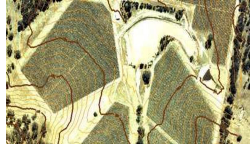
Contour superimposed on an orthophoto
