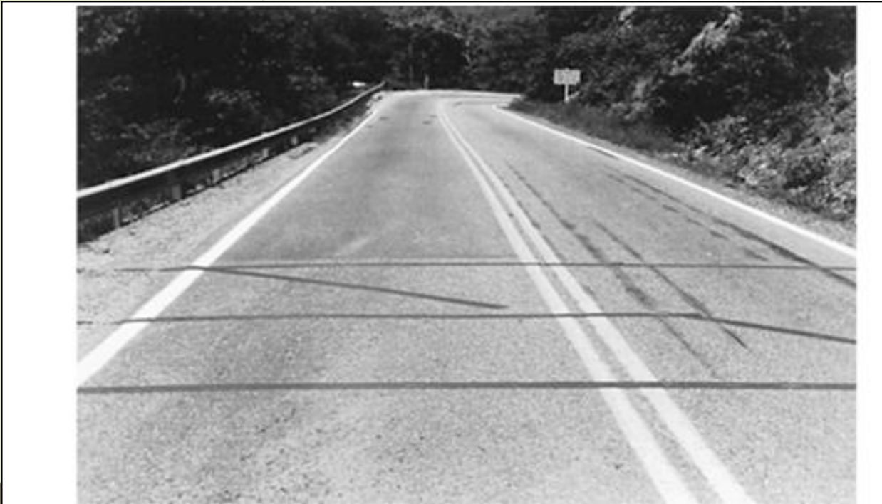
Figure 4.2 An Example of a Sensor Setup of a Surface Detector Using Pneumatic Road Tubes
