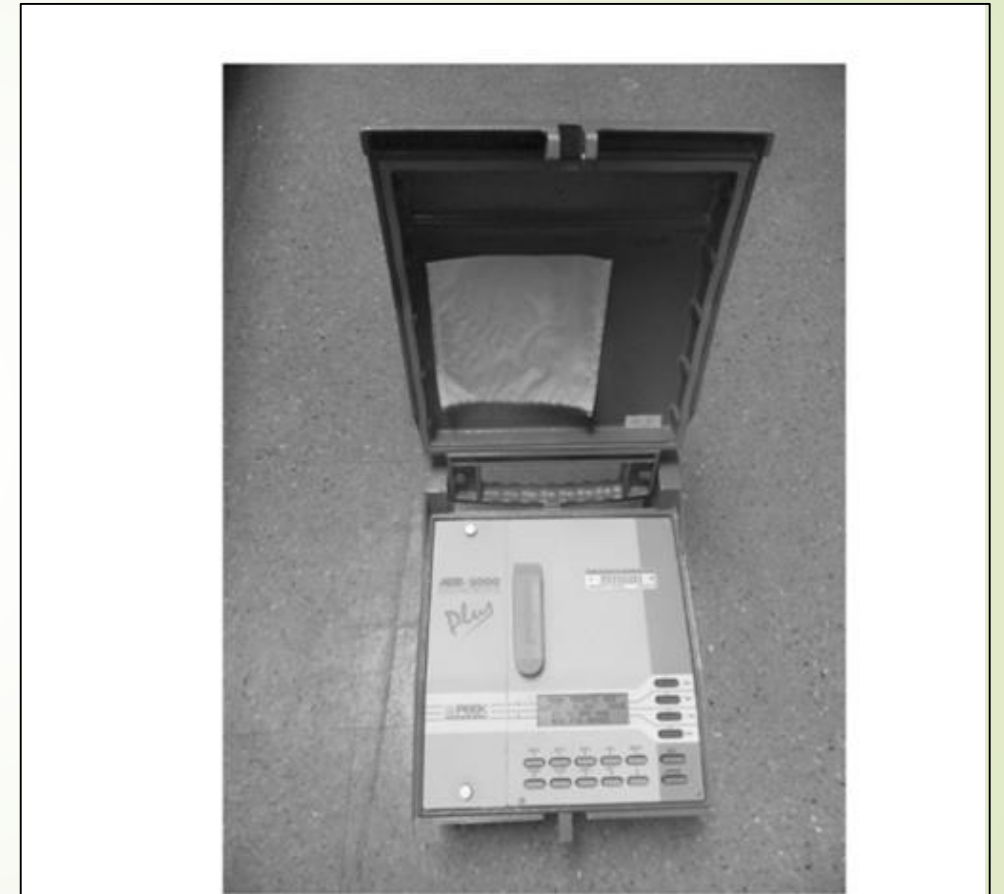
Figure 4.3 PEEK JR 161 Portable Loop Traffic Counter
