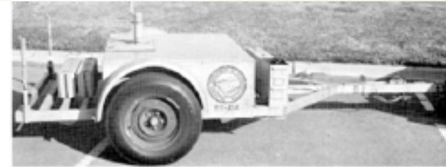
Figure 21.5 Mays Ride Meter Trailer Unit
