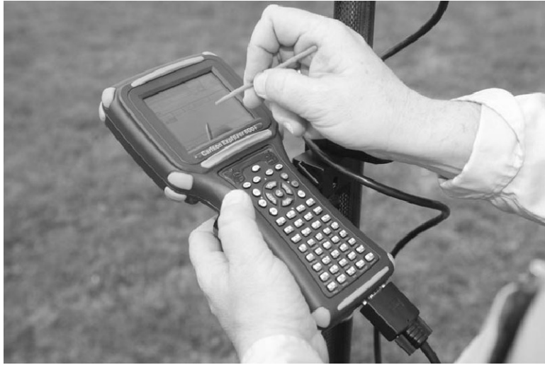
Figure 14.4(e) Carlson Explorer 600+ Digital Data Collector
