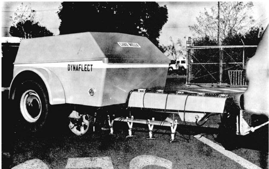
Figure 21.10 Dynaflect Deflection Sensors
