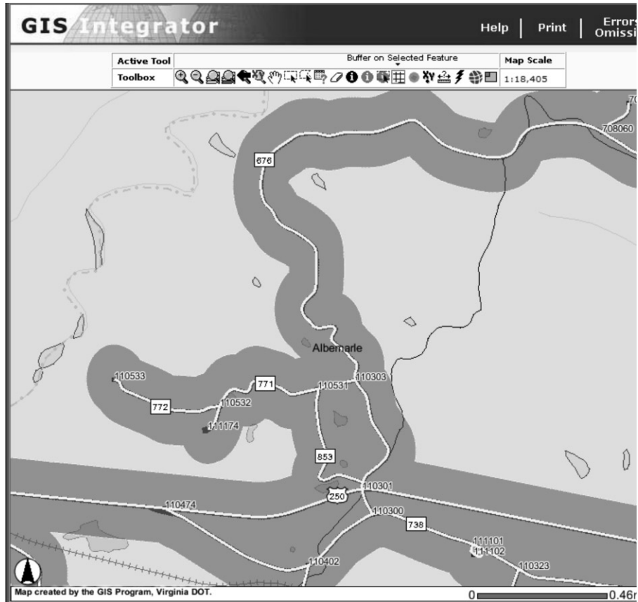
Figure 11.12 GIS Buffer Analysis to Identify Wetlands Impacted by Roadways
