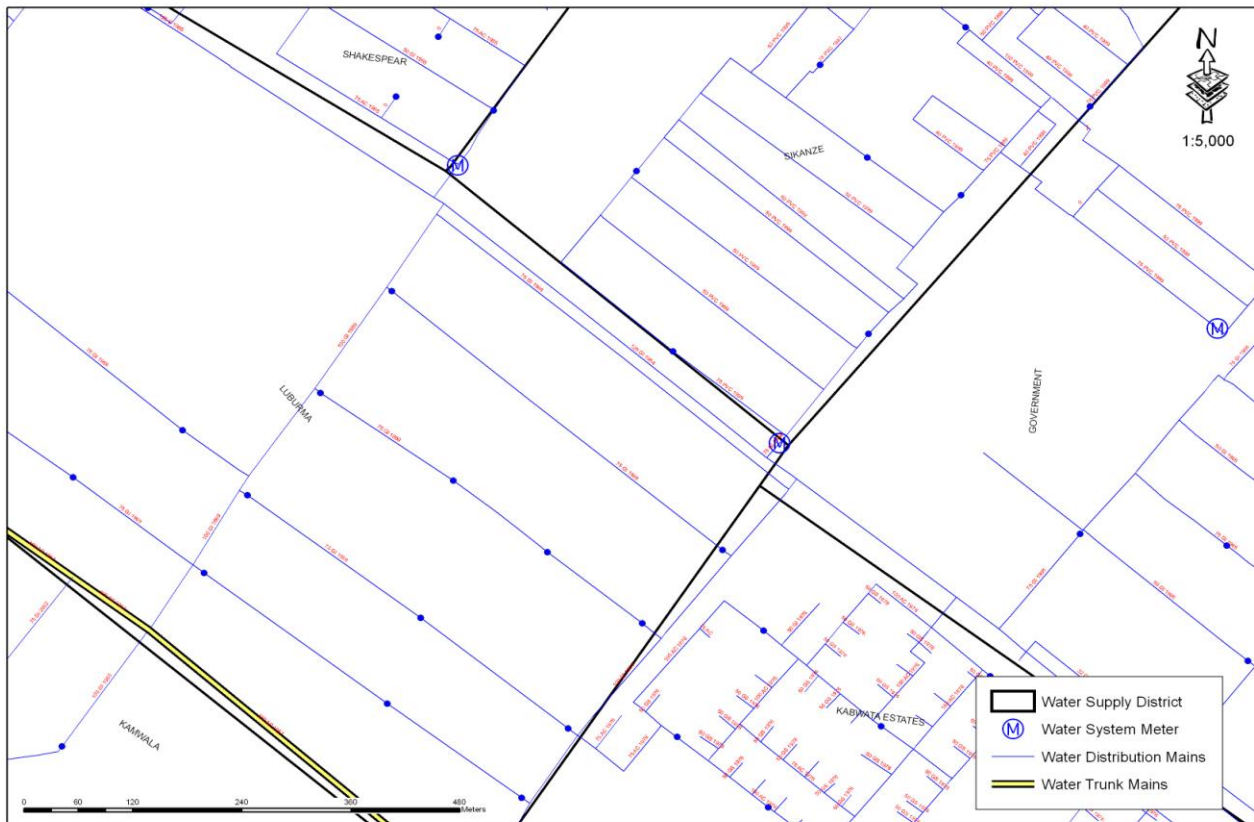
Figure 3 — Diagram of subdivisions of a water distribution system
