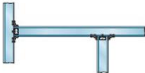
fixed-connected overhanging beam
