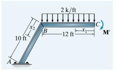
For  $x_1$ :  $M_1 = -(x_1^2 + M')$  $\frac{\partial M_1}{\partial M'} = -1$ For  $x_2$ :  $\zeta + \Sigma M = 0;$   $-M_2 - 24(x_2 \cos 60^\circ + 6) - M' = 0$  $M_2 = -24(x_2 \cos 60^\circ + 6) - M'$  $\frac{\partial M_2}{\partial M'} = -1$
