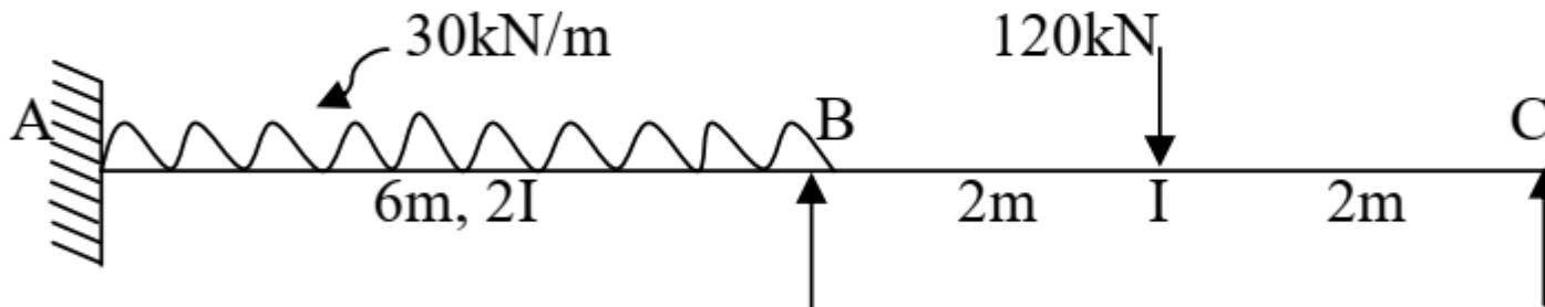
NOTE: In this case of example with sinking of supports, the redundant should be selected as the vertical reaction.
