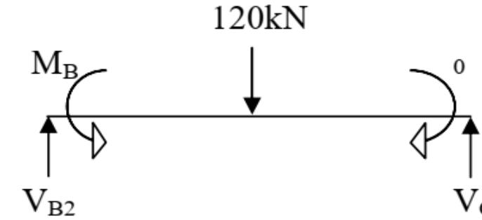
$$V_A = 96.64\text{kN}, \quad V_{B1} = 83.36\text{kN}, \quad V_{B2} = 78.07\text{kN}, \quad V_C = 41.98\text{kN}$$
