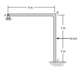
Determine the reactions at the supports, then draw the moment diagram for each member. EI is constant.
