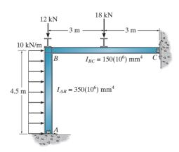
Determine the moments at the ends of each member of the frame. The supports at A and C and joint B are fixed connected. EI is constant.
