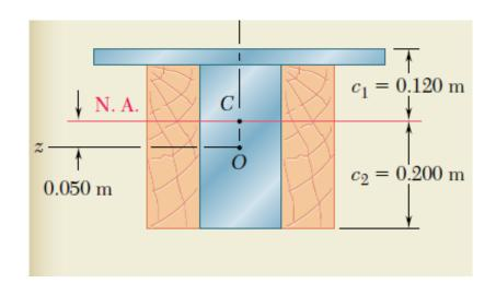
**b.** Stress in Steel. Along the top edge  $c_1 = 0.120$  m. From the transformed section we obtain an equivalent stress in wood, which must be multiplied by n to obtain the stress in steel.
