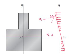
The neutral axis will be drawn *through the* centroid of the transformed section and the stress  $\sigma_x$  at any point of the corresponding fictitious homogeneous member will be obtained from  $\sigma_x = -\frac{My}{I}$
