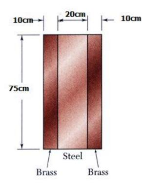
Bar is made from bonded pieces of steel ( $E_s = 200$ GPa) and brass ( $E_b = 105$ GPa). Determine the maximum stress in the steel and brass when a moment of 40 N.m is applied.
