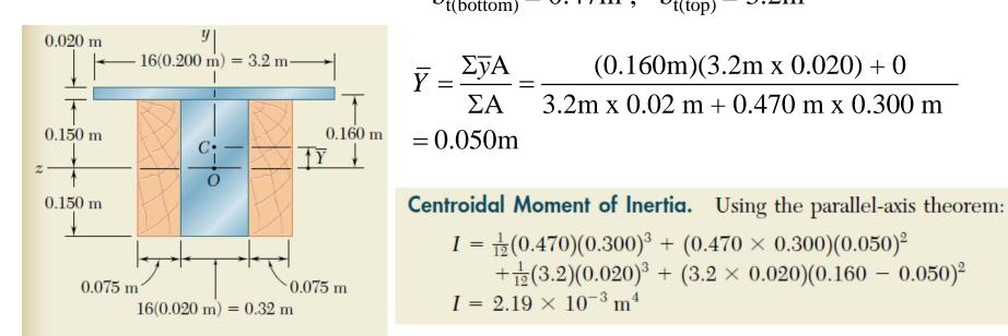
**a. Maximum Stress in Wood.** The wood farthest from the neutral axis is located along the bottom edge, where  $c_2 = 0.200$  m.
