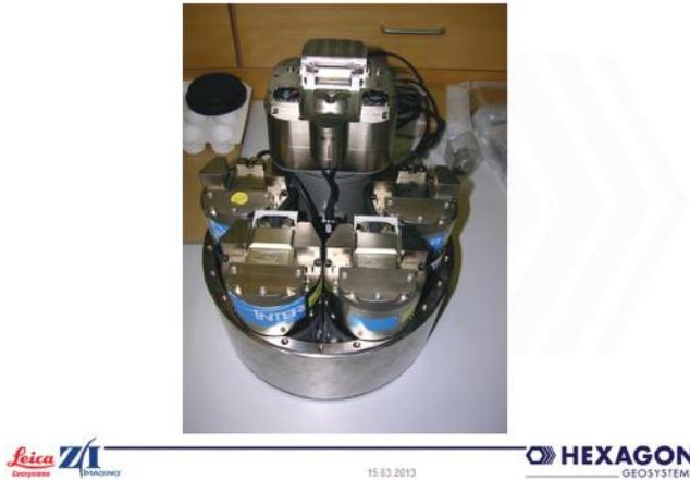
**Figure 2.22** Mounting of 5 DMC2 camera parts in frame. (From Leica Geosystems, Heerbrugg, Switzerland, for Hexagon.)
