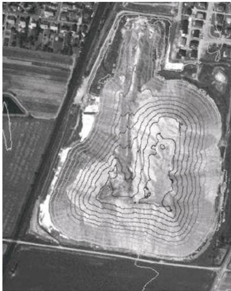
**Figure 3.89** Interpolation of contours from the TIN. (Image courtesy of the Institute for Photogrammetry and GeoInformation, University of Hannover, Germany.)
