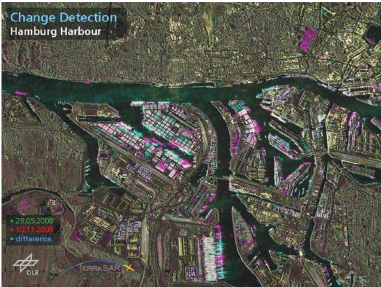
**Figure 2.64** Interferometric survey of elevation changes in Hamburg harbor, Germany. (From DLR, Oberpfaffenhofen, Germany.)
