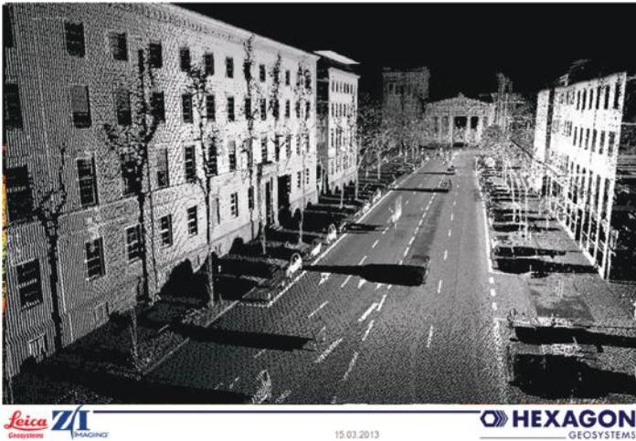
**Figure 2.26** Laser image from mobile van. (From Leica Geosystems, Heerbrugg, Switzerland, for Hexagon.)
