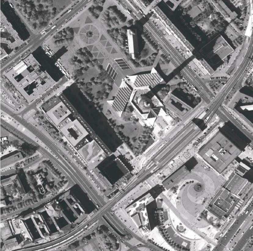
**Figure 2.50** Rectified ADS 40 image. (Courtesy of LH Systems [Leica Geosystems], San Diego, California. © Leica Geosystems, 2000.)
