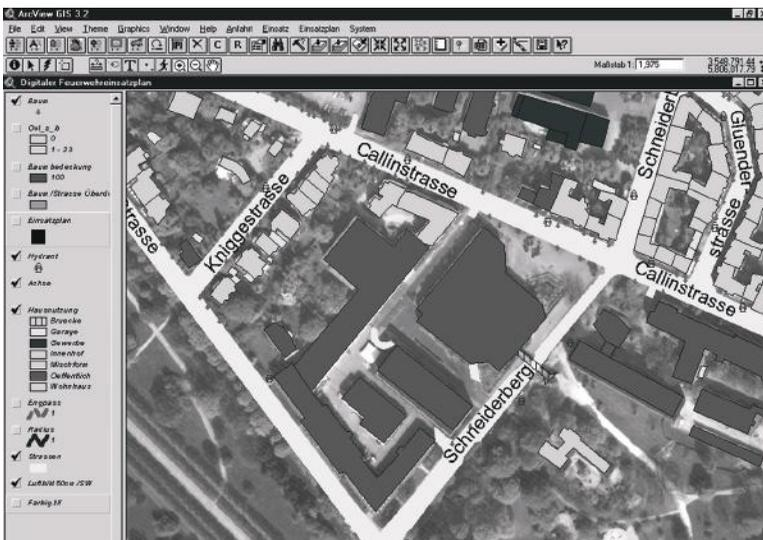
Figure 4.118 Digital orthophoto for deriving crown diameters of trees. (Map courtesy of the Institute for Photogrammetry and GeoInformation, University of Hannover, Germany.)
