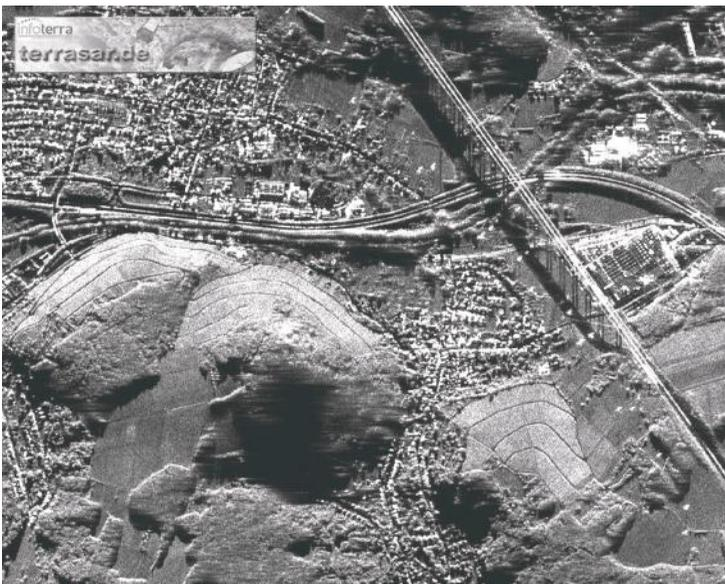
**Figure 2.61** Radar imaging distortions. (From DLR, Oberpfaffenhofen, Germany.)
