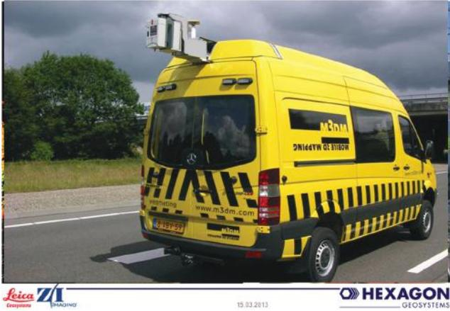
**Figure 2.25** Mobile van operation of ALS70. (From Leica Geosystems, Heerbrugg, Switzerland, for Hexagon.)
