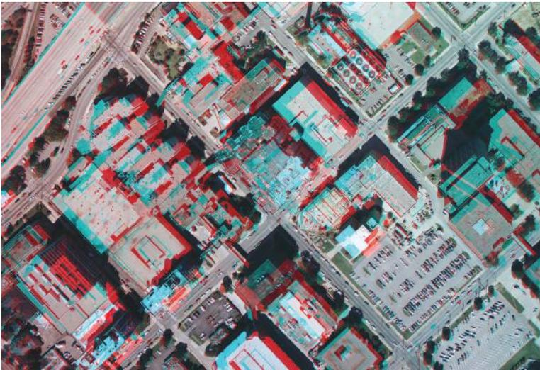
**Figure 2.79** Anaglyphic stereo view of two overlapping aerial photos of Louisville, Kentucky. (Data provider: Photo Science, Inc.; Illustration provider: ERDAS Inc., the Geographic Imaging unit within Leica Geosystems GIS & Mapping Division, Atlanta, Georgia.)
