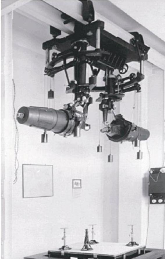
**Figure 3.25** The Gasser Projector, 1915, rebuilt by Carl Zeiss, 1933, in compact form. (From the ISPRS Archives; previously published by ISPRS for the 100th Anniversary 2010 by G. Konecny.)
