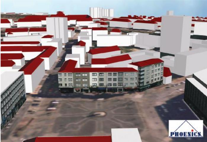
**Figure 4.126** Addition of building façade texture, orthophoto texture for the ground and derivation of roof types from DSM height differences for buildings. (Image courtesy of Phoenix GmbH, Hannover, Germany.)
