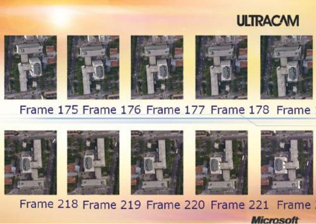
Figure 2.31 Overlapping frames. (From Microsoft-Vexcel, Graz, Austria.)
