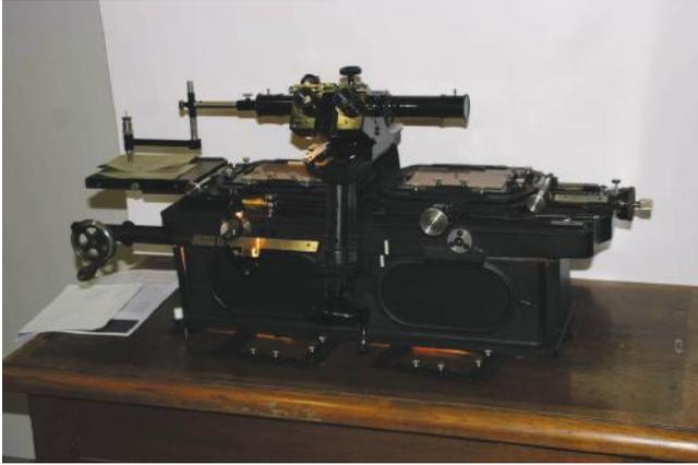
**Figure 3.14** Pulfrich Stereocomparator built by Carl Zeiss, 1901. (From the ISPRS Archives; previously published by ISPRS for the 100th Anniversary 2010 by G. Konecny.)
