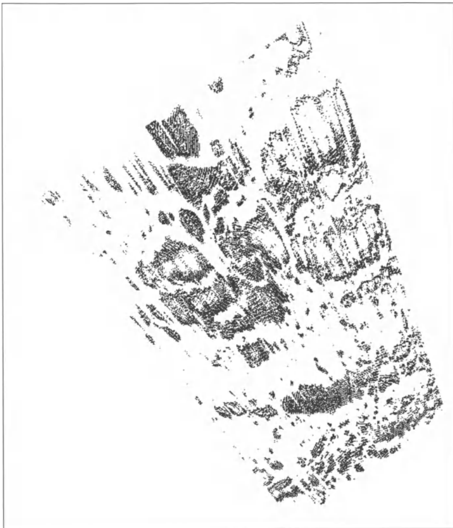
Fig. 43: Points found by correlation, showing the wave structures. The cameras are looking from bottom right.
