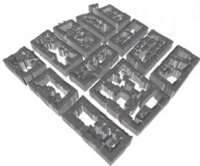
Figure 8.1-10: Building model extracted from laser scanner data
