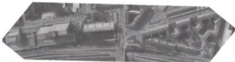
Figure 7.3-3: Orthophoto generated using a ground model 7
