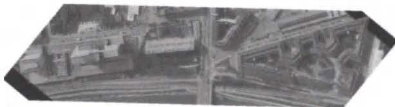
Figure 7.3-4: Orthophoto generated using a surface model which also contains buildings and man-made structures; double imaging occurs here due to the missing visibility analysis 7
